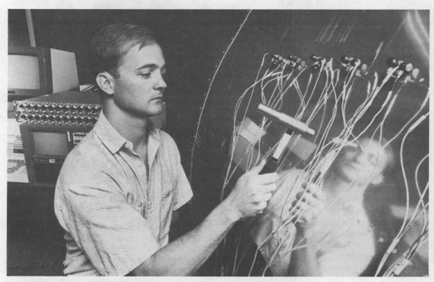
VIBRATION SIGNATURES — Dennis Roach (2741) hits a replicated aircraft fuselage with a modal impact hammer as sensors measure vibration. Vibration signatures from undamaged aircraft structures can be compared to those of damaged structures to determine the type and degree of damage.
